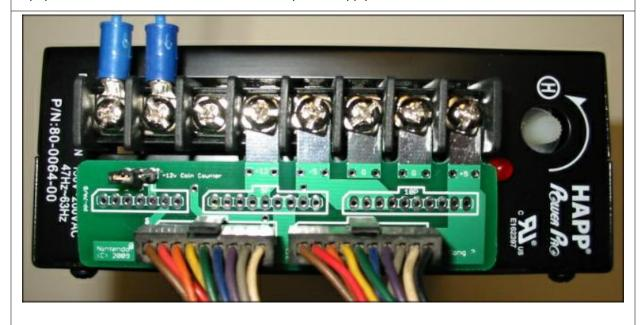
It is possible to plug your cables in backwards which will cause damage to your game boards, Ensure the tab on the connector matches the diagram on the new power supply interface adapter.
